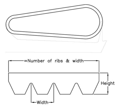
$\begin{array}{ll} \text{Datum Llength} = 698 \\ \text{Height} &= 4.45 \\ \text{Number of ribs} = 324 \\ \text{Pitch} &= 3.56 \end{array}$
